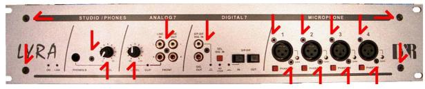
For the screws you will need a pozi drive screwdriver. To remove the pot meter nuts you will need a 11mm spanner.
