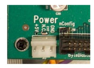
2) Now adjust the power supply so that the so that the +5V on the Core PCB is exactly +5V.
